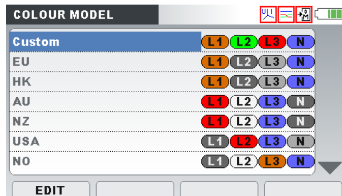
Figure 4.3: Colour representation of phase voltages
