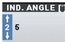
Figure 3.5: Current lags voltage by 25° angle.
