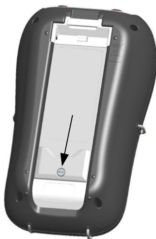
Figure 7.2: Closing the battery compartment cover
